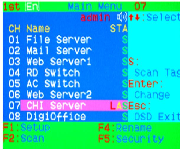
Figure 31: Lock port from the OSD main window
