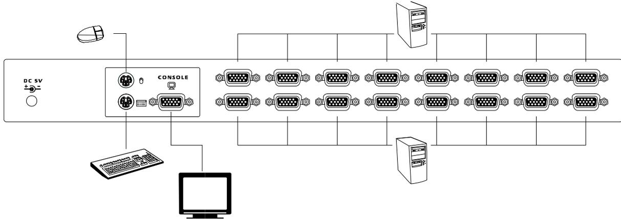
Figure 5: Console connection
